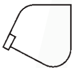
Bucket with front lip reinforcement
